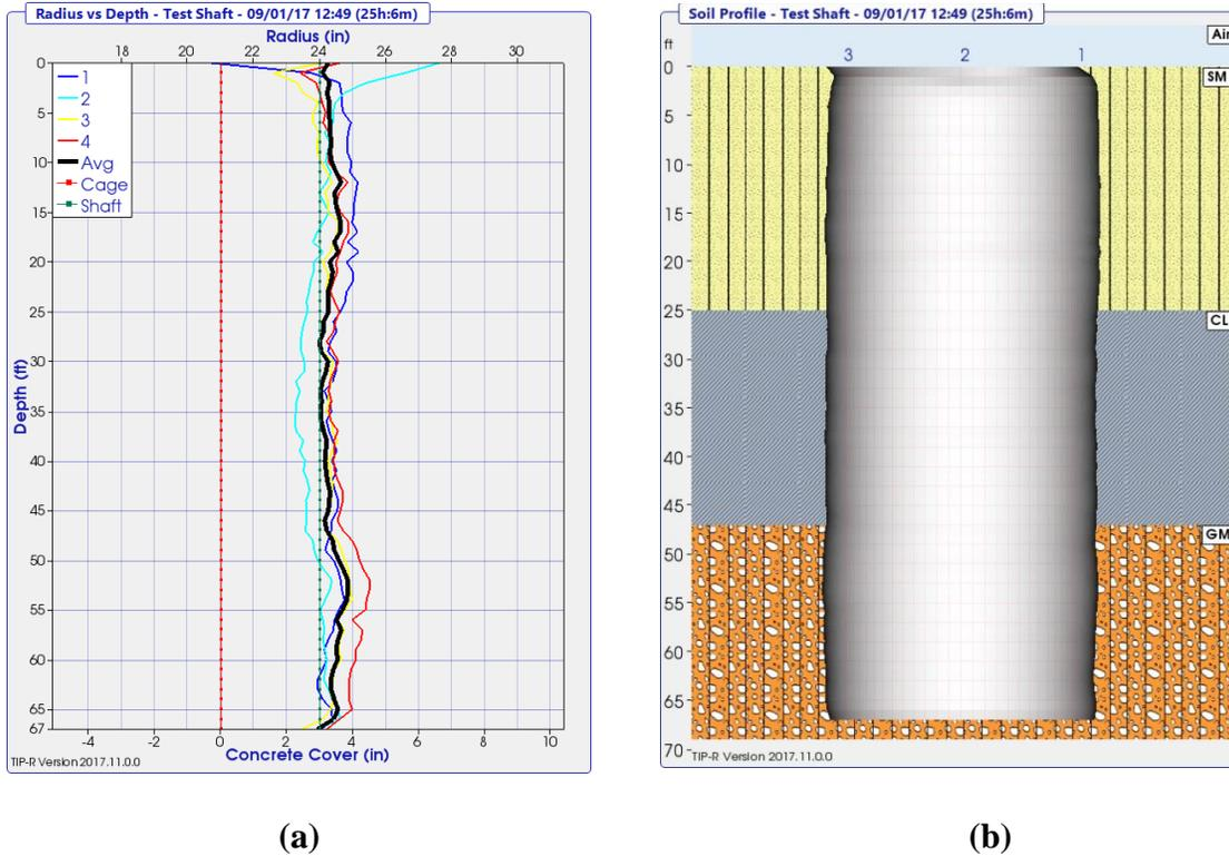
**Figure 6.** TIP results for a satisfactory drilled shaft (a) Effective Radius Vs. Depth and (b) 3D Model overlaying the Soil Profile
