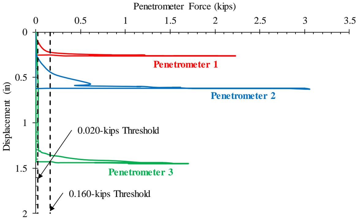
**Figure 5a.** Debris Thickness from SQUID testing, Ref. [4], Overall Thresholds
