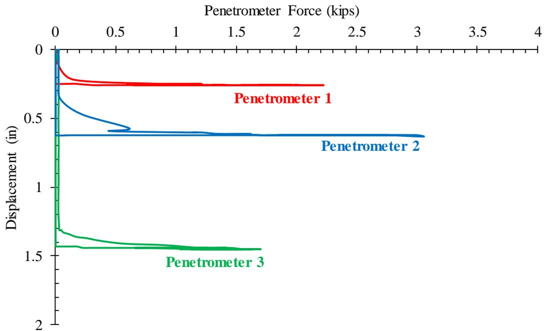
**Figure 4.** Force and Displacement plot from a SQUID Testing, Ref. [4]
