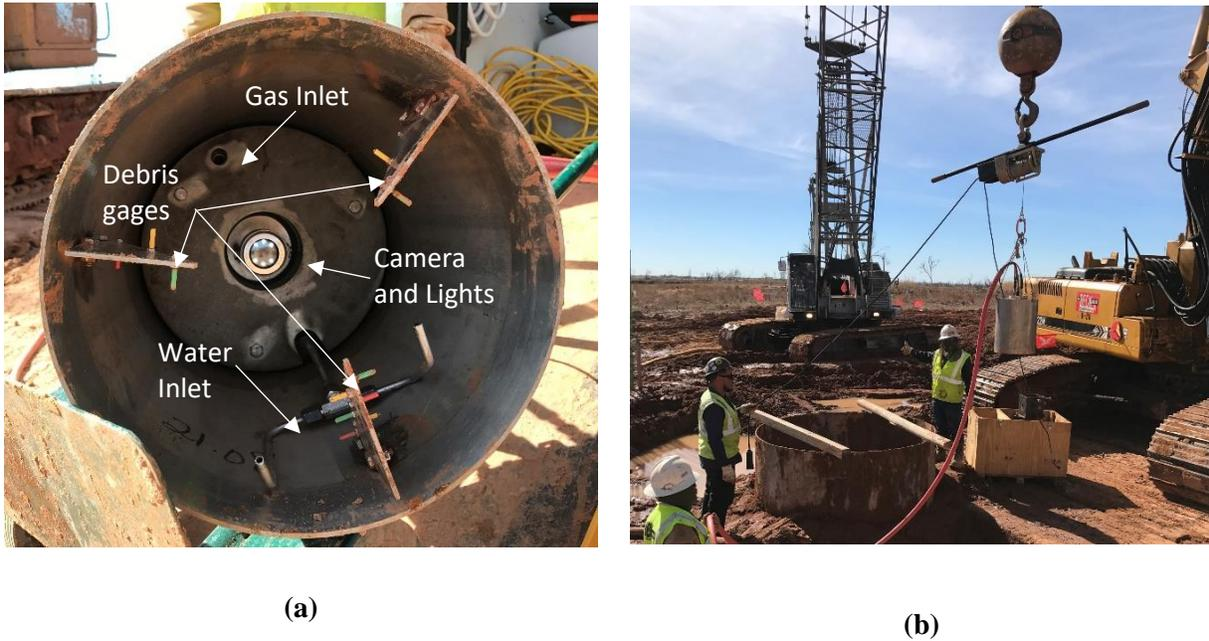
**Figure 1.** Miniature Shaft Inspection Device, Ref [4] (a) Diving Bell, and (b) Preparing for testing
