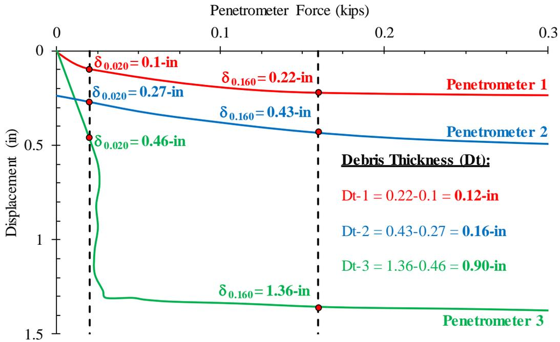
**Figure 5b.** Debris Thickness from SQUID testing, Ref. [4], Debris Thickness Calculation
